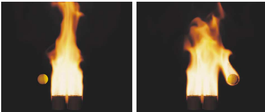
Fig. 2. The level set method allows one to accurately represent the thin flame zone that separates the unreacted gaseous fuel from the reacted hot gaseous products. This allows one to more accurately model the gaseous expansion across this interfacial zone. Here the level set method is used to simulate a ball catching on fire. For more details, see [123] where these calculations were carried out using methods first proposed in [124].
