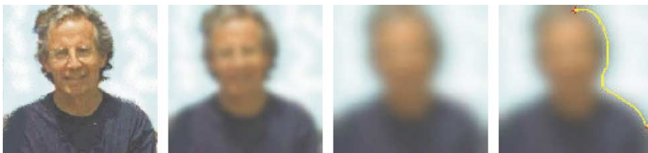
Fig. 4. Example of the heat flow (isotropic diffusion). On the left we have the original image and on the middle two different time steps of the diffusion flow, showing how the image is getting blurred. This blurring impedes the achievement of an accurate segmentation, right figure. See below for details on the segmentation technique.
